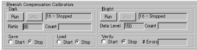
To perform calibration, first click [Run] in the [Dark] section. You will be instructed to set a particular saturation level for compensation. The process will then proceed automatically until the compensation data for dark pixels has been created. Use the [STOP] button if you want to halt the process before it is completed.
