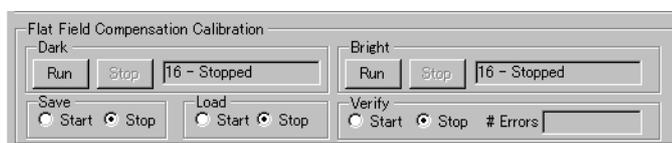
Calibration must be performed in the sequence of [Dark] first, then [Bright]. Begin by clicking the [RUN] button in the [Dark] section. A pop-up window will instruct you to close the lens before continuing. Calibration will then proceed automatically until completed. The status window next to the [STOP] button shows the percentage of completion. It can take up to 20 minutes for a calibration to be performed. Click the [Stop] button to halt the calibration at any time.
