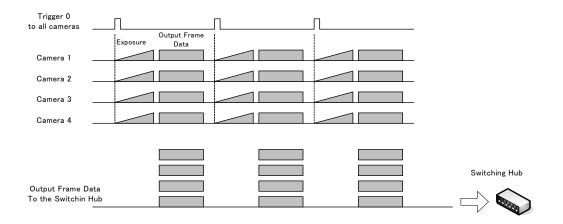
• The packet delay should be set larger. The data traffic is controlled by the buffer of the hub. It is necessary to check the buffer value of the unit.
