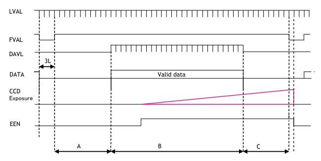
Values for vertical timing in partial scan continuous mode.
