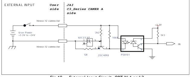
Fig.10. External Input Circuit, OPT IN 1 and 2
