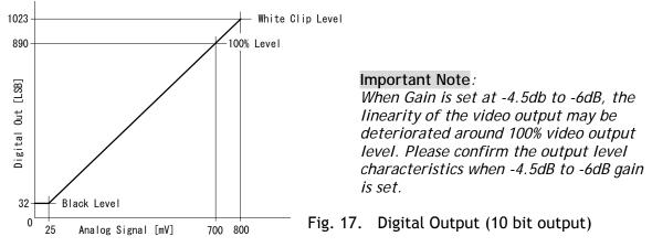
7.4.2 Bit Allocation (Pixel Format / Pixel Type) - BM-141GE (monochrome)
