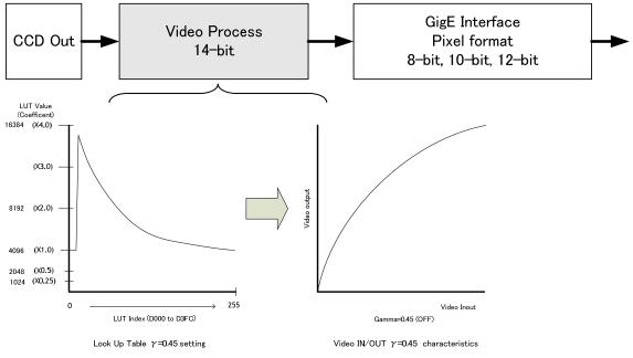
Fig.28 Setting example of Gamma=0.45
