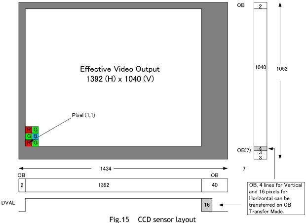
Important Note: By using Optical Black (OB) transfer mode, the user can select whether to include optical black pixels in the image stream. This is for Horizontal only.
