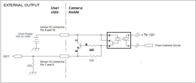
5.5.2 Recommended External Output circuit diagram for customer
