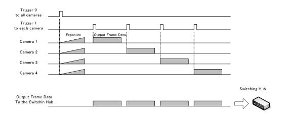
• The packet delay should be set smaller, and the packet delay trigger controls the data traffic. If the camera has a pulse generator, it can control the data traffic.
