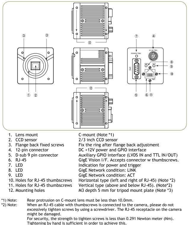
\*3) Note: The tripod adapter plate MP-41 can be used with BM/BB-141GE
