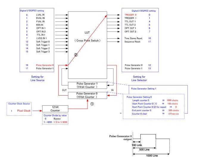
Fig.14 Pulse Generator 0 timing Example 2
