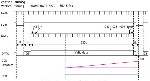
Fig.24 Vertical Timing for Vertical Binning
