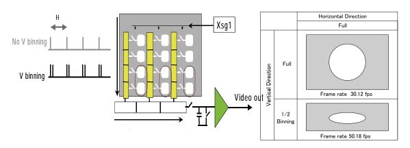
Fig. 16. BM-141GE Vertical binning.
