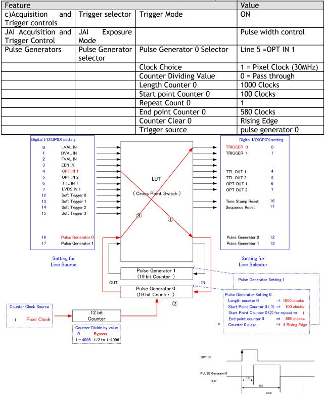
Fig.13 Pulse Generator Timing Example 1
