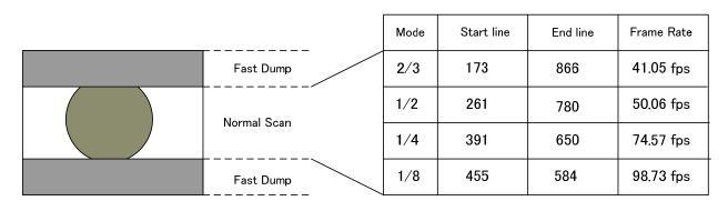
In addition to the mentioned fixed rate partial scan modes, BM/BB-141GE has variable partial scan mode. The start line can be set from 1st line to 1025 line and the scanned lines can be set from 8 lines to 1032 lines. Please note that if the odd line is selected as the start line, the Bayer color sequence is RGR and if the even line is selected, it is GBG.
