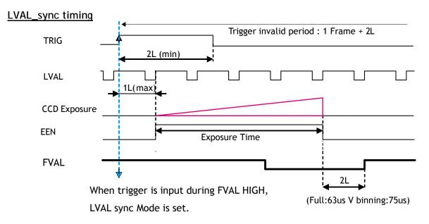
Fig. 28 Edge Pre-select LVAL sync Timing
