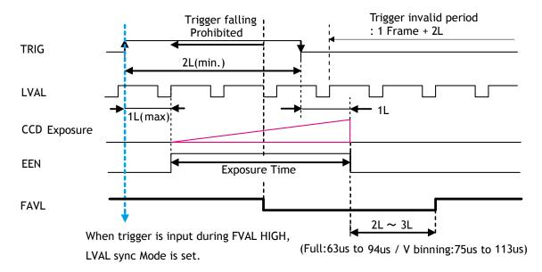
Fig. 31 Pulse width control LVAL sync.
