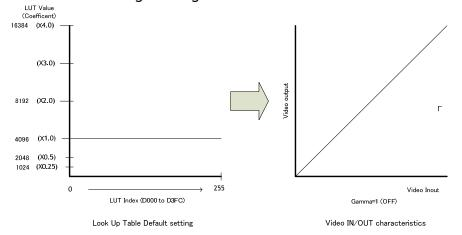
Fig. 27 LUT default setting (Coefficient: x1.0=4096)
