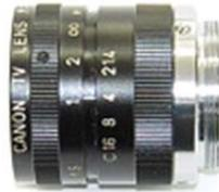
5. Under this condition, rotate the lens. As the flange back adjustment ring is rotated simultaneously, set the ring so as to focus the lens. (①).
