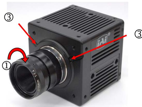
1. Attach the C mount lens to the camera (①).
