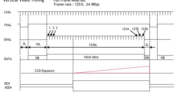
Fig. 17. Vertical timing for full scan
