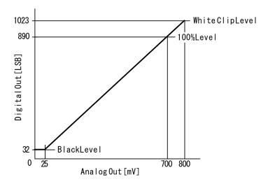
Fig.9. Digital Output Bit Allocation
