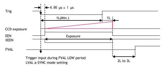
Fig. 25. Pulse Width trigger mode. LVAL asynchronous
