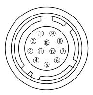
Fig. 3. Hirose 12-pin connector.
