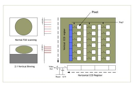
Fig.14. Vertical Binning
