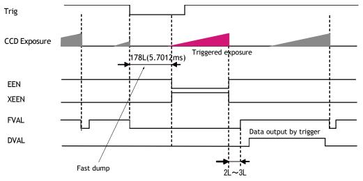
Note: When PE is set at 1251 or the shutter is set at OFF, EEN is always HIGH.
