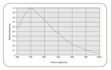
Fig. 30. Spectral Response for CM-200MCL/PMCL
