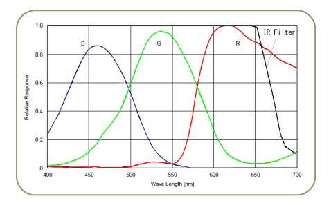
Fig. 31. Spectral Response for CB-200MCL/PMCL
