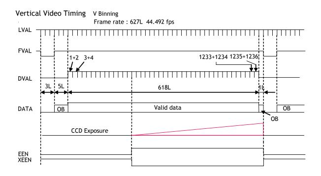
Fig.21. Vertical Timing for Vertical Binning
