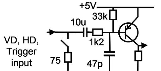
Fig. 5. HD, VD and Trigger input.
