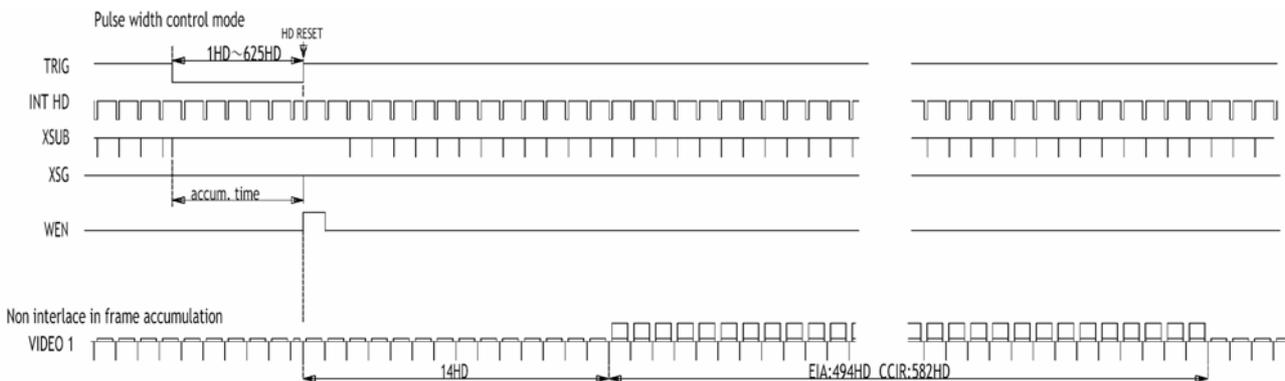
Fig. 17. Pulse width control. H reset
