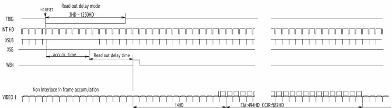
Fig. 19. Frame delay read out. H reset
