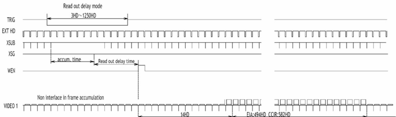
Fig. 18. Frame delay read out. H non-reset
