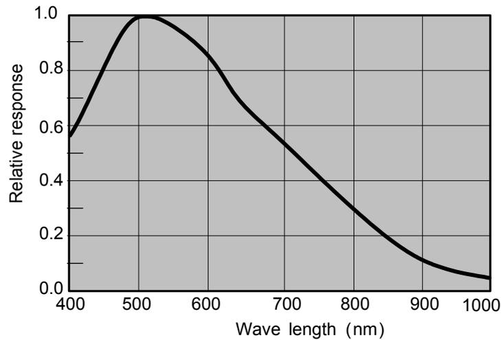
Fig. 26. Spectral sensitivity for CV-M10SX
