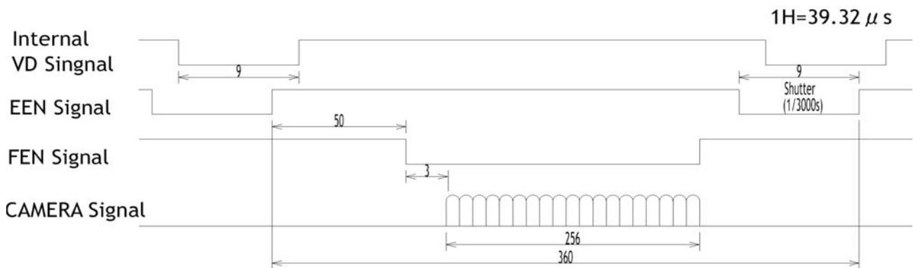
Fig. 18A. Vertical timing details with 1/4 partial scanning.
