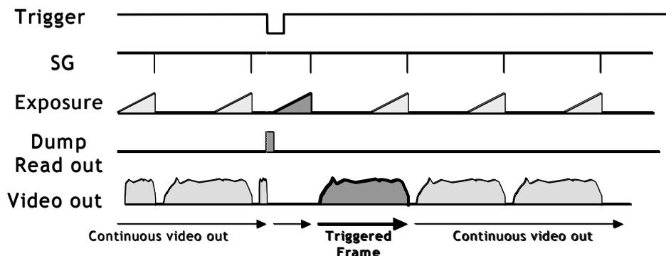
Fig. 15. Restart Continuous Trigger mode.
