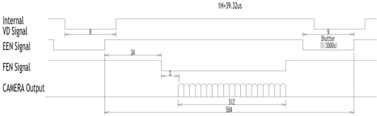
Fig. 18. Vertical timing details with 1/2 partial scanning.
