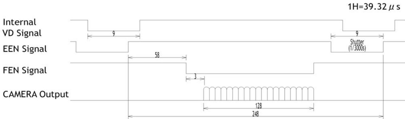
Fig. 18B. Vertical timing details with 1/8 partial scanning.
