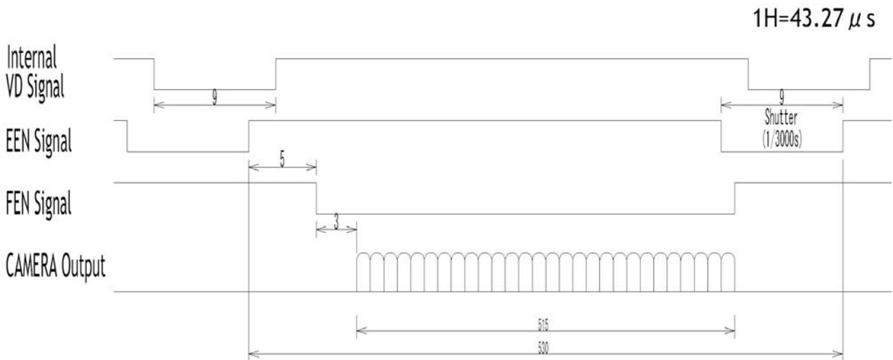
Fig. 17A. Vertical timing details with vertical binning (M4<sup>+</sup> and M4<sup>+</sup>CL only).
