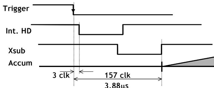
Fig. 19. Accumulation latency time for H a-synchronous trigger.
