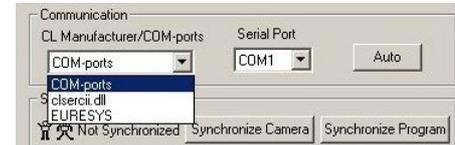
Just select the option for the frame grabber that is installed in the pc.
