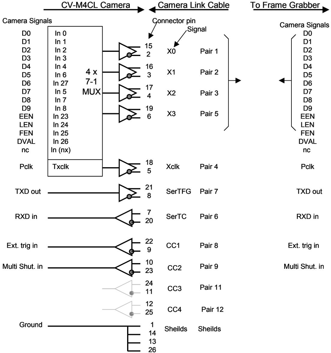
Fig. 8. Principle diagram for Camera Link interface
