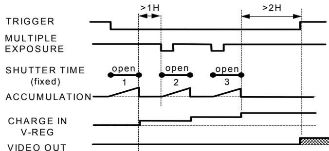
Fig.13. Multiple exposure
