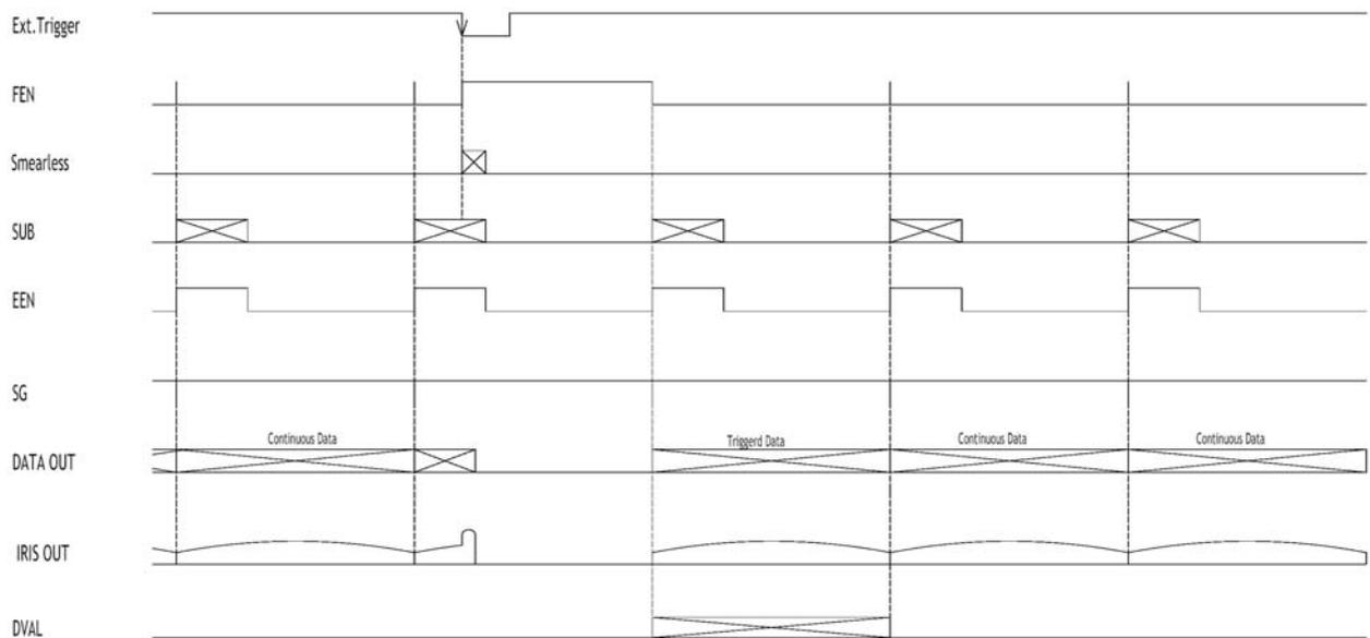
Fig. 21. Edge Pre-select with Restart Continuous Trigger.
