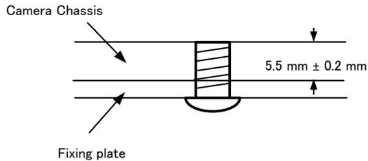
Fixing the camera on the plate
