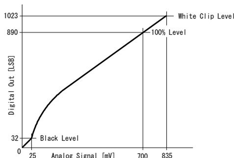
Fig.18 LUT characteristics
