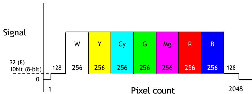
Fig. 16 Color bar test pattern
