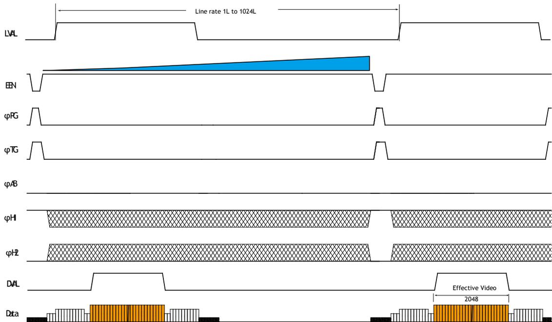
Fig.12 No-Shutter mode with internal line rate generator
