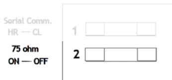
Fig. 21 Rear panel DIP-switch
