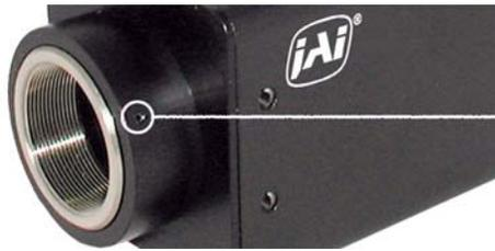
Loosen the three 2mm screws around the perimeter of the C-mount lens collar (two 2mm screws for a CS-mount) to adjust the back focus. Unless you absolutely must, do not attempt to adjust this focus.
