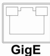
Use at least Cat5e UTP cables (Cat6 cables are preferred). JAI recommends the use of shielded cables to reduce emissions and for CE/FCC compliance. Double-shielded cables further reduce emissions.
