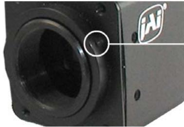
Loosen the three 2mm screws around the perimeter of the C0mount lens collar (two 2mm screws for a CS-mount) to adjust the back focus. Unless you absolutely must, do not attempt to adjust this focus.
