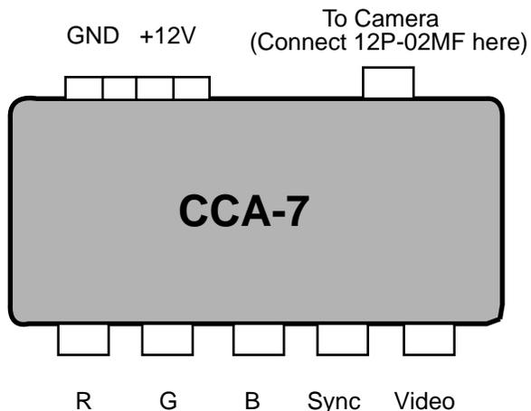
Note: RGB option is only available when TMC-73M is modified for use with CCA-7. Contact PULNiX for further assistance.
