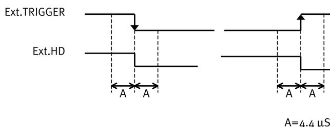
3. The ext. trigger input is TTL level. The duration should be more than 1 H negative going. >64  $\mu$ sec. and < 60 msec. The input is AC coupled.
