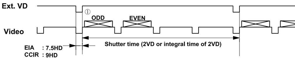
**c) Non interlaced mode (Field accumulation mode)**
