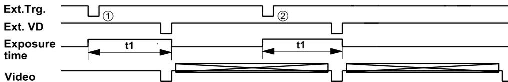
**b) 2:1 Interlaced mode (Field accumulation mode)**
