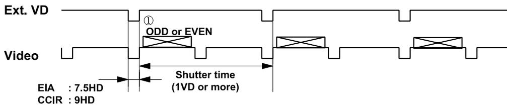
**b) 2:1 Interlaced mode (Frame accumulation mode)**
