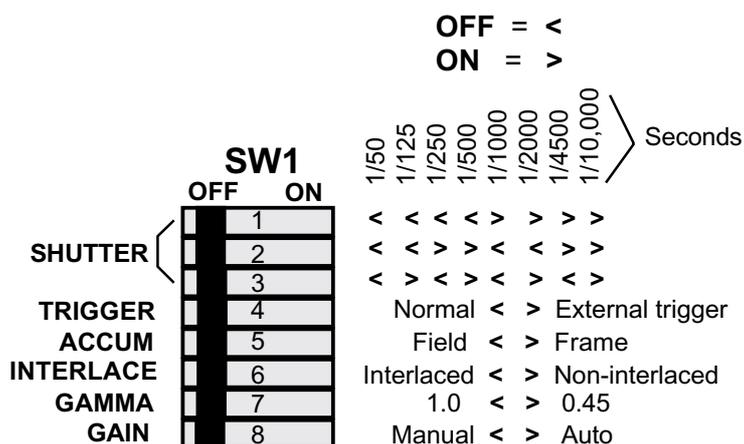
The shutter values are given for a CCIR camera having the factory settings. Shutter values for other setups and EIA cameras can be seen in table 7.1.3.
